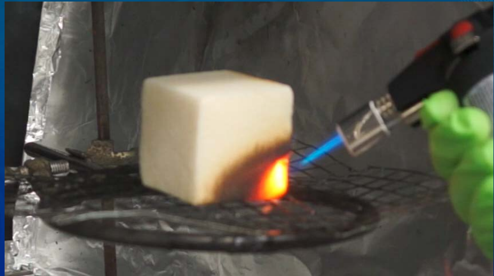
Treated Polyurethane Foam sodium polyborate - clay additive
