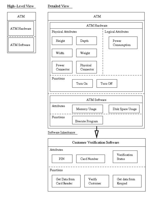
Figure 12. High-level, detailed, and software inheritance views of system structure and hardware/software system breakdown for an ATM Machine (adapted from Austin [2002]).
