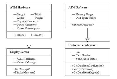
Figure 15. UML system structure diagrams for hardware and software components.
