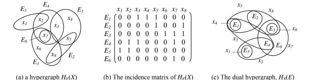
Figure 2. A hypergraph, its incidence matrix and its dual (Adapted from Berge 1989)
