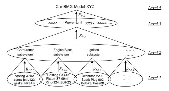
Figure 19. A car represented as a multilevel assembly system – a systems of systems
