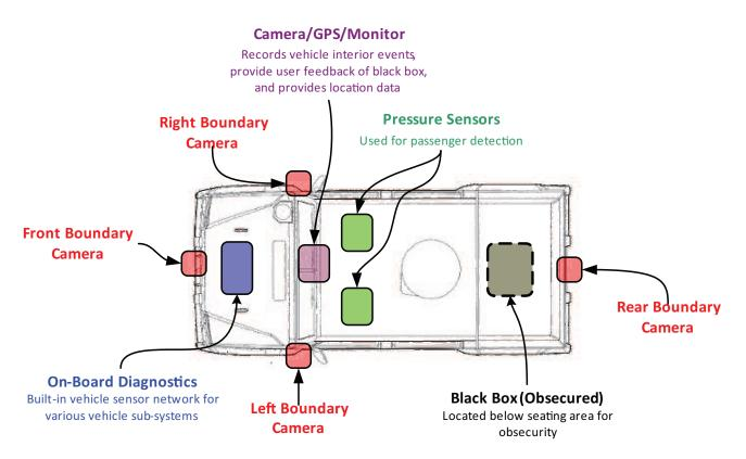
Figure 2.3: Complete Black Box system layout diagram showing the location of each subsystem
