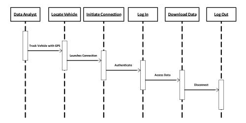
Figure 4.8: Sequence Diagram of Retrieving Data
