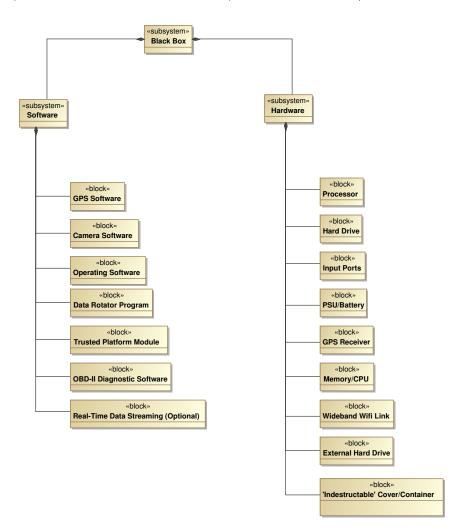
Figure 6.2: Black Box Structure Diagram
