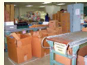
After: shorter conveyors, less prone to queue.
