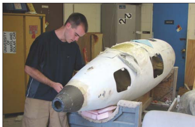
Above: ME undergrad James Michael prepares the human-powered submarine fiberglass shell for competition in 2007.
